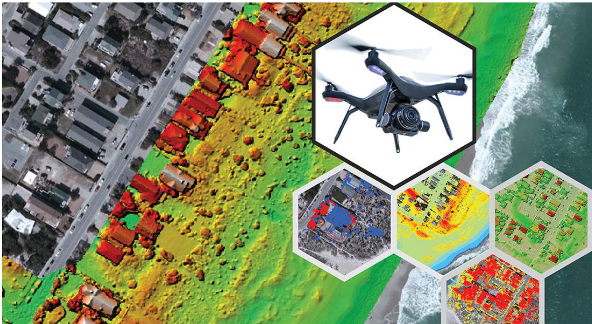
Figure 3.6. The imagery demonstrates the feasibility of using drones to replace or augment surveys using high-resolution 3D mapping. The drone is a 3DR ® Site Scan with a Sony ® R10C camera. Images courtesy of 3D Robotics ® . Drone image courtesy of McKim & Creed.
