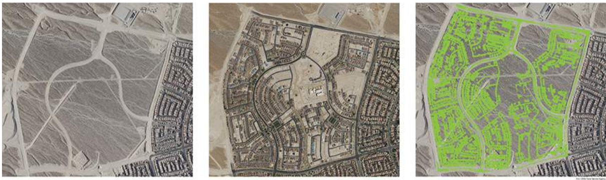
Figure 5.1. This area in Las Vegas, Nevada, highlights urban change detection between two dates using National Agriculture Imagery Program (NAIP) imagery. The green thematic layer was created from a change detection process and is overlaid on an older image to show where change occurred.
