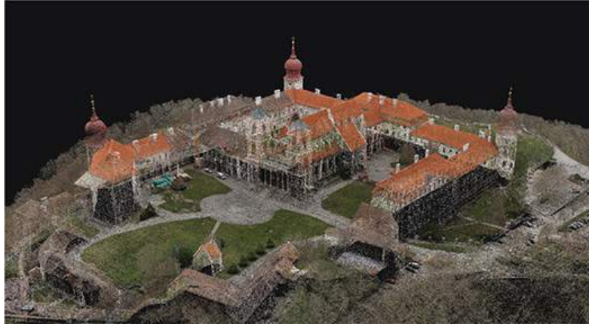
Figure 5.16. Lidar image showing points being used to extract a building—Goettweig Abbey, Austria. Courtesy of RIEGL®.
