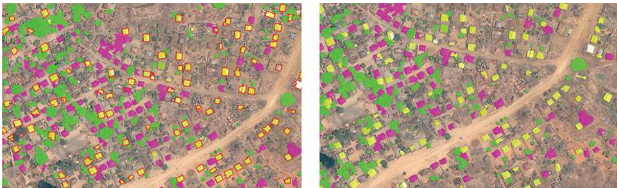
Figure 5.8. Image analytics example. A trained dataset showing various samples used to extract different roof types in Mozambique.
