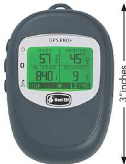
Figure 3.7. The Bad Elf GPS Pro + is a Bluetooth GPS + GLONASS receiver and data logger, accurate up to 2.5 meters. It quickly acquires satellite lock without cell tower assistance.
